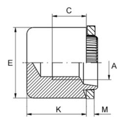
Female thread A = M10Height K = 14.0Min thread length C = 6.0Outer diameter E = 19.0Plate thickness = 3.8 to 4.0
